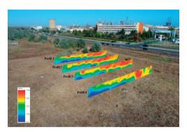
Figure 4. Apparent resistivity sections - Perimeter I
