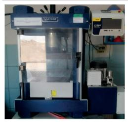
Figure 3. Matest 2000KN concrete press
