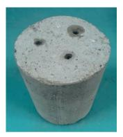
Figure 2. Pre-drilled soil sample
