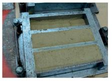
Figure 3. Casting fresh clay mixture in metal moulds
