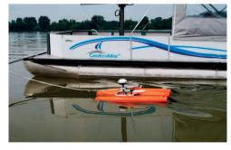
Figure 2. Multiparameter probe, model EX02 and the PAH probes, microFlu from Aquams and ADCP River Ray 600 kHz
