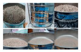
Figure 6. Size sorting of shredded ceramic waste
