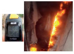
Figure 9. Complete combustion of the ETICS on the side wall to the fire compartment
