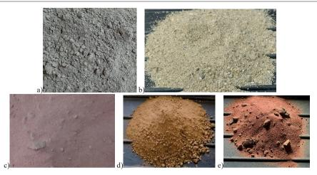
Figure 4. Raw materials: a) Portland Cement; b) Natural sand (0/4), S; c); SG 1 (Source 1 (ISIM), sampling: April 2022); d) SG 3 (Source 1 (ISIM), sampling: August 2023); e) SG 5 (Source 2 (Tim Cut SRL), sampling: 2023)
