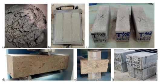
Figure 7. Specimen preparation and testing: a) fresh state aspect of the mortar during mixing sequences; b) fresh mortar casted in the prismatic mold; c) SG 5 50% mix specimen after removal from the mold, 24 h after casting and specific conditioning (air, high moisture (>95%)); d) Specimen placement in the 3PB testing equipment; e) Compression testing; f) Specimens after 3PB and compressive testing
