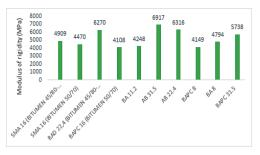
Figure 4. Graphical representation of the modulus of rigidity
