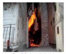
Figure 10. Burning particles detached from the thermal system
