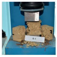
Figure 8. Compressive strength of the prism halves
