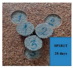
Figure 6. Appearance of the SP1R1T coating, containing rice husks and hemp fibers, and the way it breaks when pulled off, for determining adhesion at 28 days
