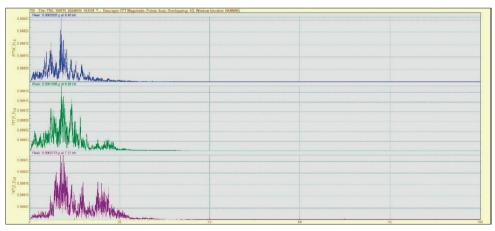
Figure 10. FFT magnitude plots for the FOC6 ground motion record. Event: 16.09.2024 Vrancea earthquake
