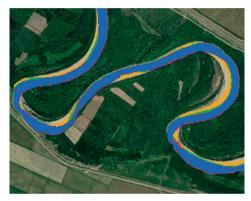
Figure 7. Water bodies dynamics between 2016-2025 based on NDWI Index (orange - 2016, green - 2019, red - 2022 and blue - 2025)
