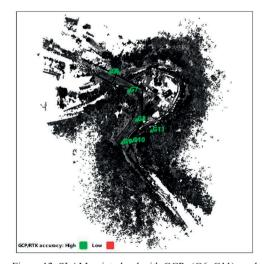
Figure 12. SLAM point cloud with GCPs (G6–G11) used for spatial alignment and accuracy validation in the national coordinate system
