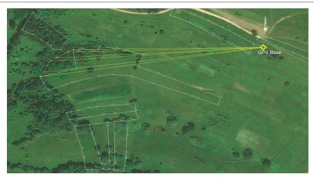
Figure 6. Positioning of plots occupied by forest vegetation using the RTK method, with radio modules
