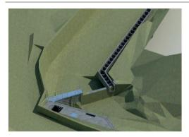
Figure 13. 3D rendering of the rehabilitated water intake structure, designed based on topographic and LiDAR measurements, showing the restored weir, retaining walls, and access elements integrated into the terrain
