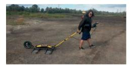
Figure 6. Georadar acquisition data with 100MHz antenna
