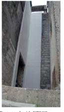
Figure 3. Test stand with ETICS prepared for fire resistance testing generated from the fire compartment
