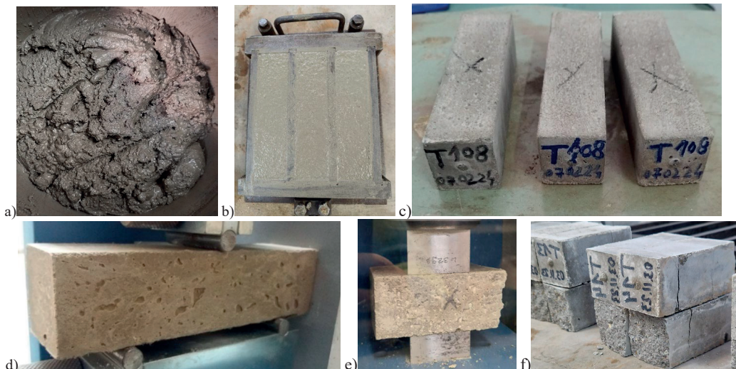
Figure 7. Specimen preparation and testing: a) fresh state aspect of the mortar during mixing sequences; b) fresh mortar casted in the prismatic mold; c) SG 5 50% mix specimen after removal from the mold, 24 h after casting and specific conditioning (air, high moisture (>95%)); d) Specimen placement in the 3PB testing equipment; e) Compression testing; f) Specimens after 3PB and compressive testing
