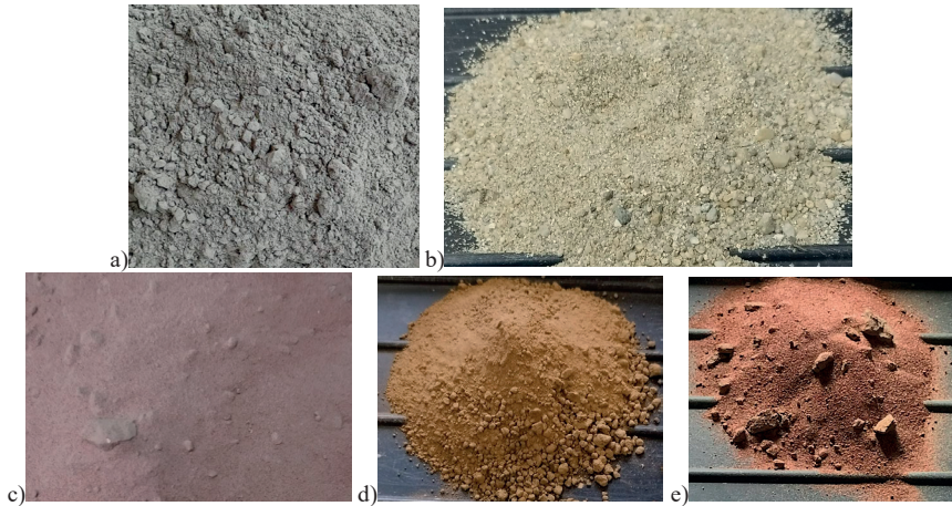
Figure 4. Raw materials: a) Portland Cement; b) Natural sand (0/4, S); c) SG 1 (Source 1 (ISIM), sampling: April 2022); d) SG 3 (Source 1 (ISIM), sampling: August 2023); e) SG 5 (Source 2 (Tim Cut SRL), sampling: 2023)
