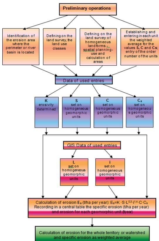
Figure 3. Organising operations to estimate sheet erosion
