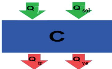
Figure 2. Greenhouse heat balance model
