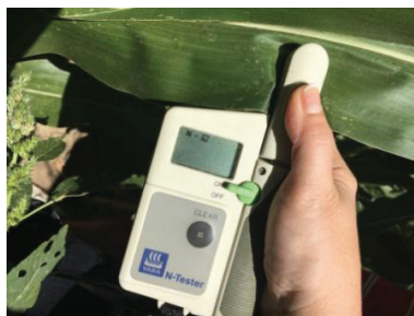
Figure 1. N Tester measurement procedure
