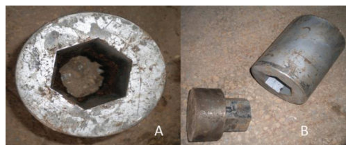
Figure 1. (A) Die for hollow-core hexagonal briquettes with the centered shaft; (B) die for full hexagonal briquettes
