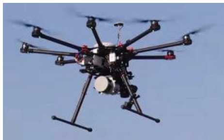
Figure 1. Unmanned aerial vehicles (UAV) with LiDAR, INS and GNSS
