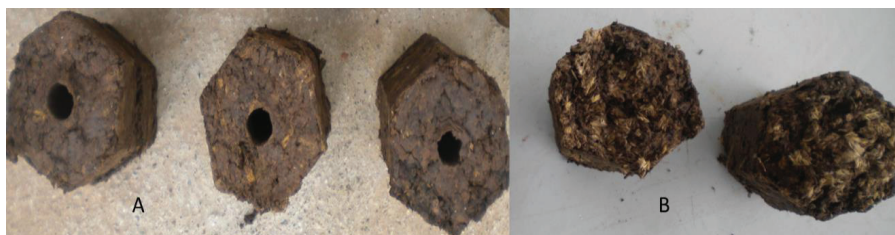
Figure 2. (A) Hollow-core hexagonal briquettes; (B) full hexagonal briquettes
