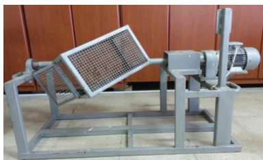
Figure 3. Durability tester for briquettes in experiments
