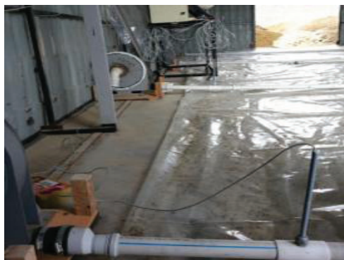
Figure 9. Airflow measurement unit
