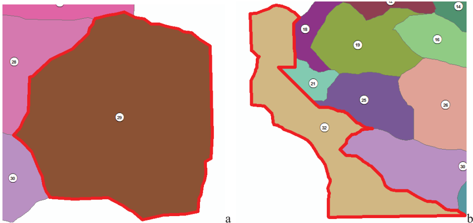
Figure 9. Circularity coefficient (a. minimum, b. maximum), Ferencz et al., 2016
