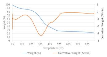
Figure 5. TG and DTG curves for full hexagonal briquettes
