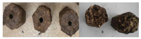
Figure 2. (A) Hollow-core hexagonal briquettes; (B) full hexagonal briquettes
