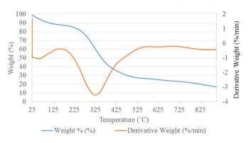
Figure 4. TG and DTG curves for hollow-core hexagonal briquettes
