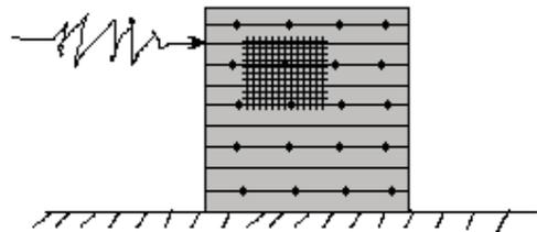
Figure 9. Reinforced and confined masonry with polymer grids subjected to earthquake
