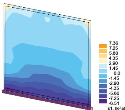
Figure 10. Displacement diagram for confined and reinforced masonry ( $T = 0.22s$ ), normal stress ranges (kPa)
