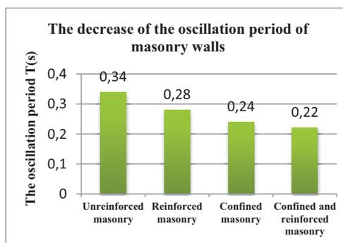
Figure 12. The decrease of the oscillation period of masonry walls
