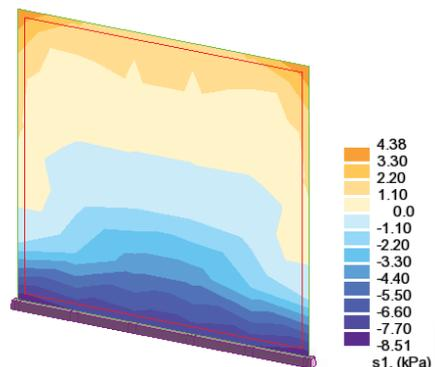
Figure 4. Displacement diagram for unreinforced masonry ( $T = 0.34s$ ), normal stress ranges (kPa)
