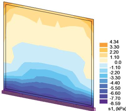
Figure 6. Displacement diagram for reinforced masonry (T = 0.28s), normal stress ranges (kPa)
