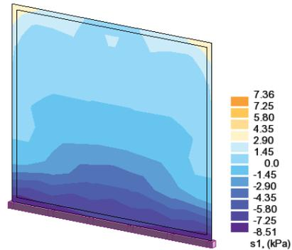
Figure 8. Displacement diagram for confined masonry (T = 0.24s), normal stress ranges (kPa)
