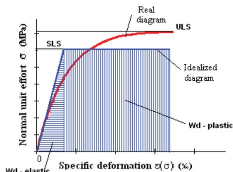
Figure 1 –  $\sigma$ - $\epsilon$  masonry curve
