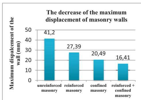
Figure 11. The decrease of the maximum displacement of masonry walls
